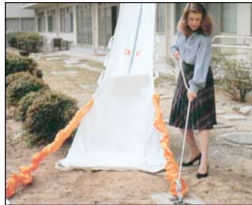
Hitch the catch to anchor point and pull out block line to extend the bag
